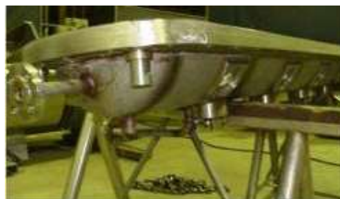
Continuous moving equilibrium reactor – Copyright Arkéma
