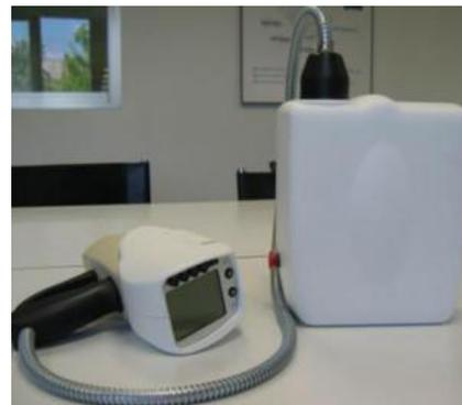
*Prototype for a portable pollutant analyser, the outcome of the Idealibs project. Copyright: Bertin Technologies*
